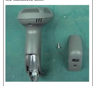
**Step 3.** Insert the battery. Leads the cable going through the groove.
