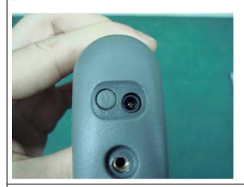
**Step 6.** Screw the screw until the bottom cover is secured.
