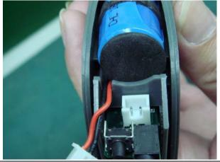
**Step 4.** Plug the battery connector into PCB socket.
